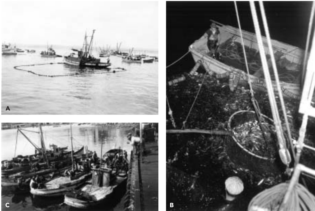
FIGURE 22-1 The Pacific sardine fishery off Monterey. (a) Setting lampara net. Photo credit: Maritime Museum of Monterey. (b) Brailing sardines from purse seine onto fishing vessel. Photo credit: Maritime Museum of Monterey. (c) Sardine-laden vessels tied up to cannery dock. Photo credit: Maritime Museum of Monterey.
